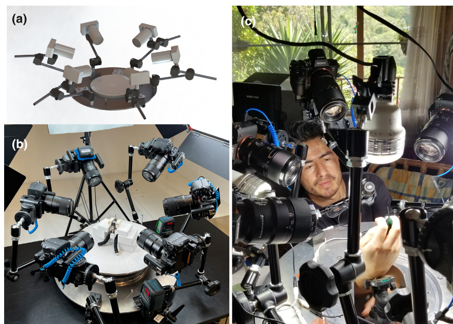
FIGURE 1 (a) A 3D CAD mockup of PicoCam, showing six cameras attached via articulating arms to a metal baseplate, facing a rotating platform that will contain the specimen. (b) PicoCam assembled indoors at the Centro Colibrí Gorriazul. LED lights have been attached to PicoCam to assist with illumination. (c) In this 'inverted' set-up, the cameras and lights rotate around the specimen.
